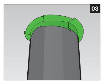
Apply Rissan around circular parts in layers
